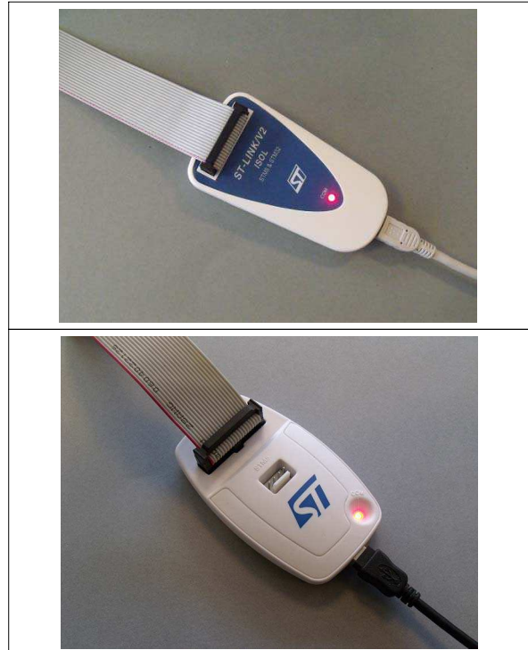
1. The first figure at the top shows the ST-LINK/V2-ISOL, while the second figure shows the ST-LINK/V2.
