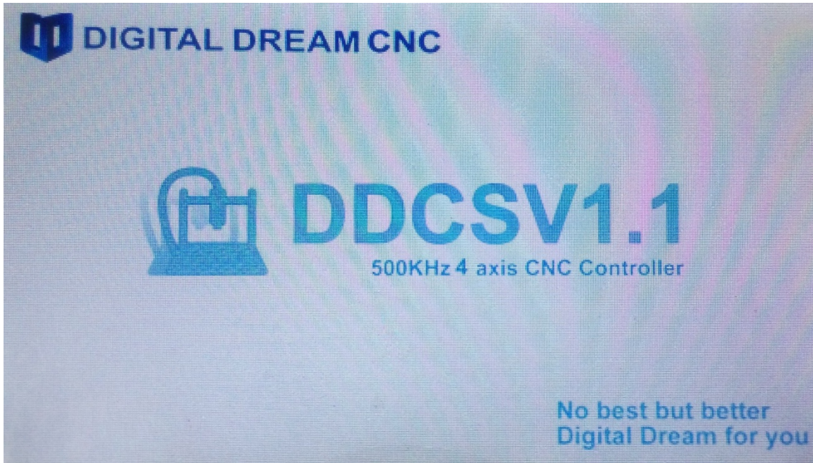
Picture 3-72 During the upgrading process, its needs to wait for 30s.
